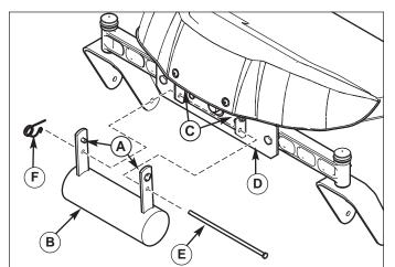
Figure 1. Install Counter Weight
